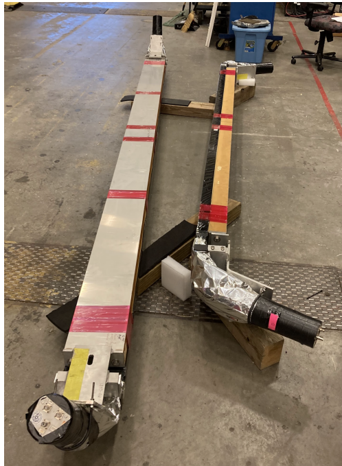
Figure 45: Cosmic paddles used for cosmic muon triggers in HCal. There are two paddles and PMTs per set, the larger of which is situated on the top of HCal in Hall A for SBS experiments.
